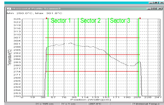
After the extruder: temperature profile with Automatic Sector and Sub-Sectors
