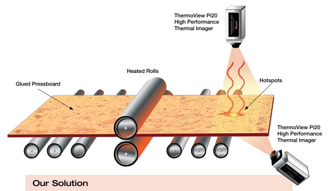
■ Raytek® ThermoView Pi20 High Performance Thermal Imager and DataTemp® DTPi Software
