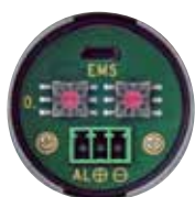
Thermalert 4.0 supports 2-wire loop
